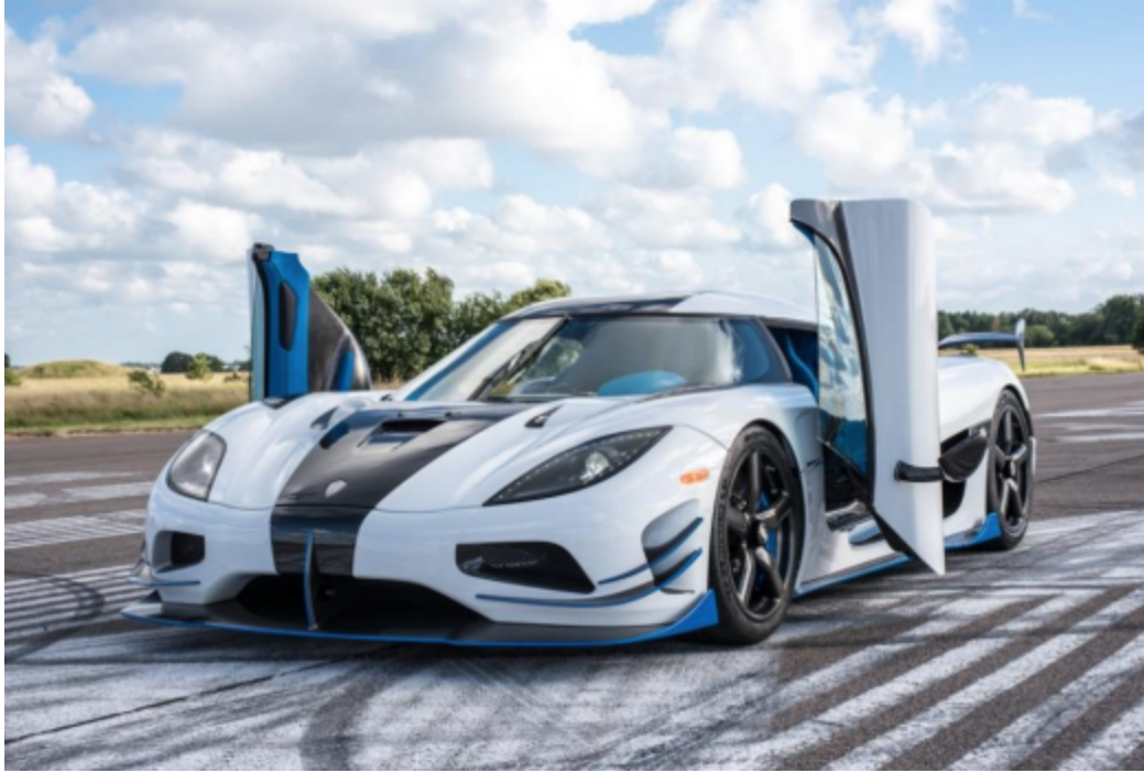
Figure X: Koenigsegg One showcasing Dihedral Synchro-Helix Actuation Doors
