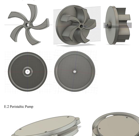
Both pumps were not chosen due to the complexity of the design: both have parts that would have had to be manufactured either using a CNC machine, which is costly, or 3d printing, which is unreliable for a fast spinning motor.
