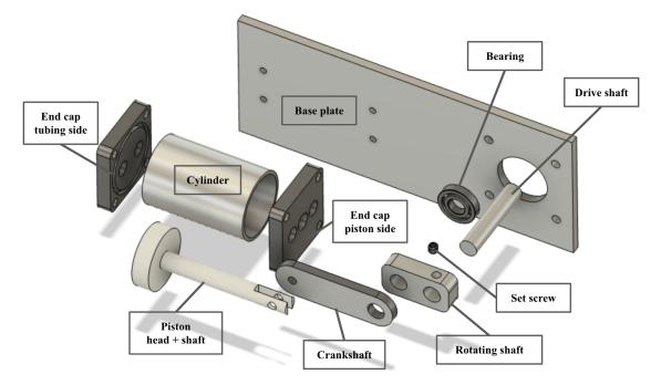
Hardware included in the exploded view are the set screw that secures the drive shaft onto the rotating shaft, and the bearing that enables smooth rotation of the drive shaft that connects the pump to the sprocket. Hardware simply for mounting were not included in the view.
