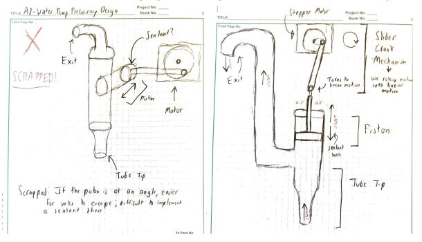
Below are the final sketches of the pump that was made.
