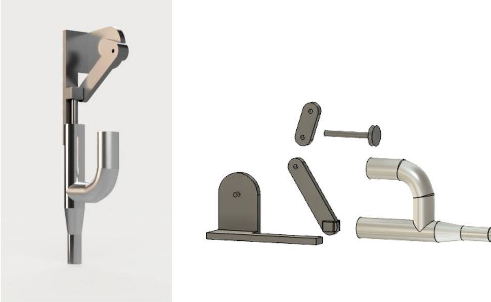
Below are the rendered and exploded views of the pump's final design.
