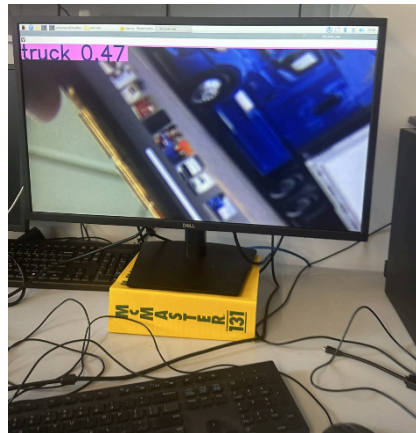
Figure 2: Initial testing of the CV algorithm running in real time with the integrated system. The lens were too focused, hence the probability of a truck detection was only 0.47.
