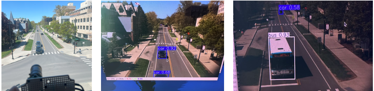
Figure 6a, 6b, 6c: Testing at Duffield Hall. Figure 6a on the left shows the testing setup, Figure 6b in the middle shows the algorithm running at moving cars in real time, and Figure 6c on the right shows the bus being detected moving in real time. All the vehicles detected are with high confidence displayed due to a well tuned and correctly oriented camera.
