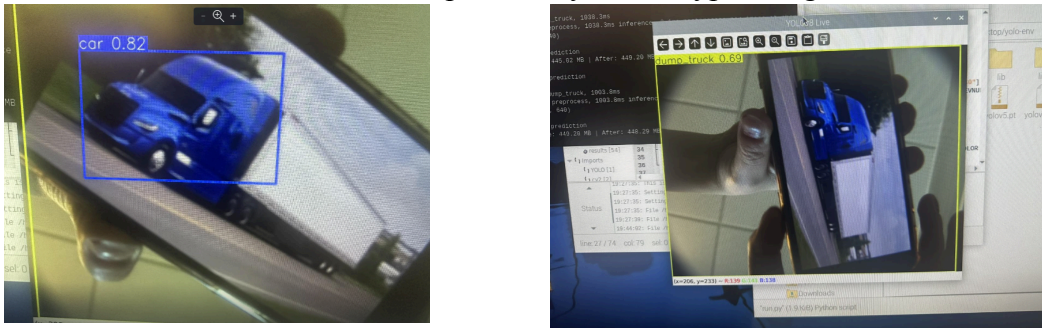
Figure 4a (on the left): The CV algorithm detecting a car due to the incorrect focus and orientation of the lens. Figure 4b (on the right): The CV algorithm detecting a dump truck with a low probability due to the orientation being inaccurate by a 90 degree shift.
