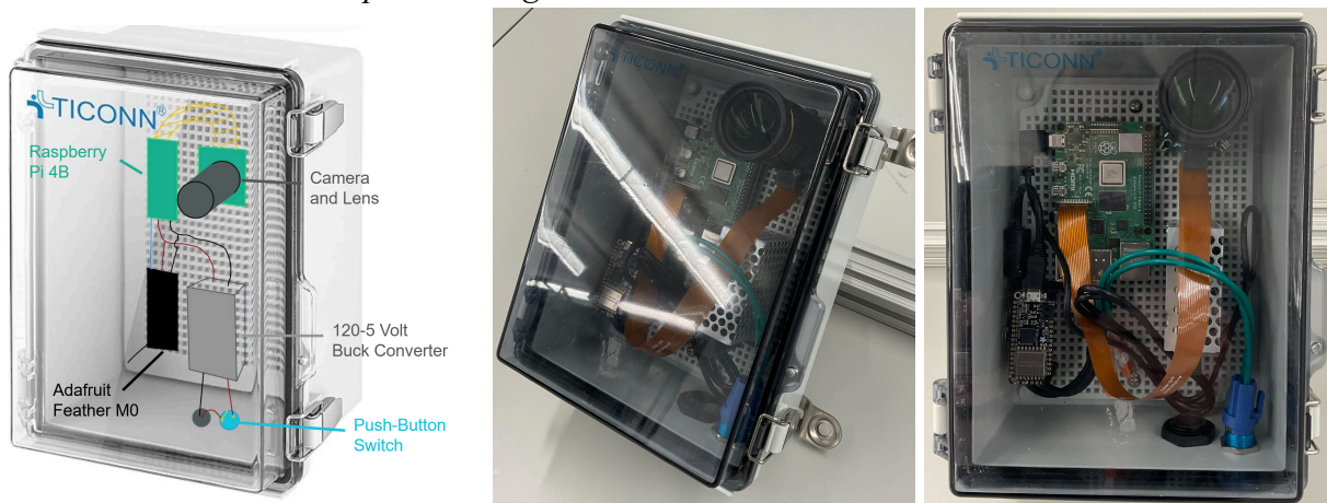
Figure 8: The enclosure (prototype sensing package) including the mounted AC-DC buck converter and the pushbutton switch. The picture on the right shows the blue pushbutton switch integrated onto the enclosure, as well as the black wire input enclosure for the incoming power line wires into the AC-DC buck converter.
